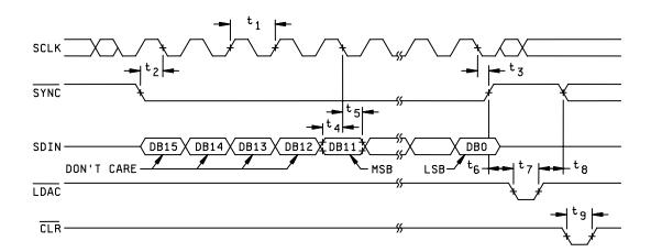
FIGURE 2. <u>Timing waveforms</u>.
